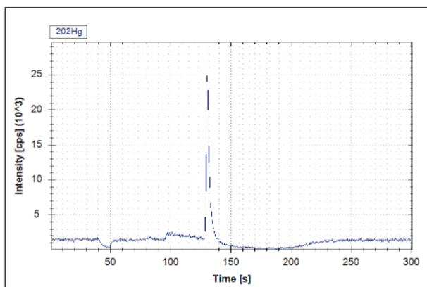
Figure 4: 0.5% NaCl solution with a 1.3 ng/g thiomersal spike.
