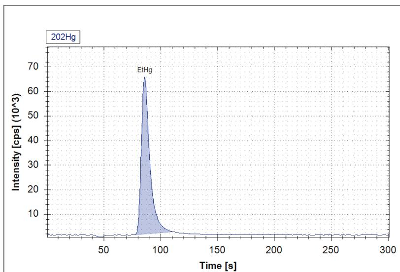
Figure 3: Chromatographic separation of  $Ethg^+$  derived from thimerosal hydrolysis.
